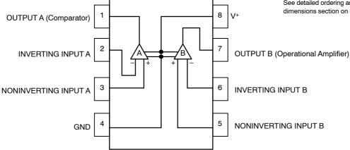
Figure 1. Logic Diagram and Pinout
